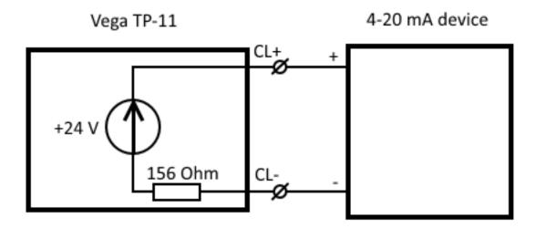
To save the battery life of the converter, the 24 V supply voltage is not continuously supplied. The 24 V voltage is applied to the 4-20 mA device a few seconds before the polling is performed so that the sensor can turn on and set the current corresponding to the measured parameter. This time, the so-called "startup time", is a configurable parameter from the configurator and can be set from 1 to 60 seconds.
