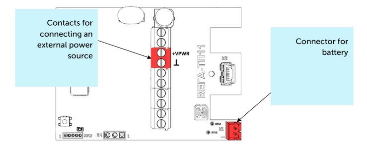
7. When the power is connected at the first time the device automatically switches to the "Active" mode and starts registration in the network. But if the device with connected battery or an external power has been switched to the "Storage" mode (by the pressing on the start button more than 5 sec) then you need to press the button to start.
